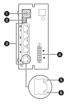
Figure 3. Rear Panel of FX82051 Module (SC Fiber Connector Shown)
